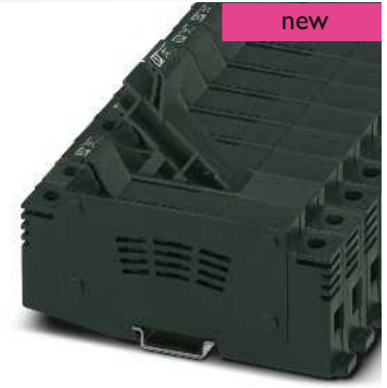
25 (25) mm 2 , 32 A, 1500 V, lever-type fuse terminal block for midget fuses 10.3 x 85 mm
