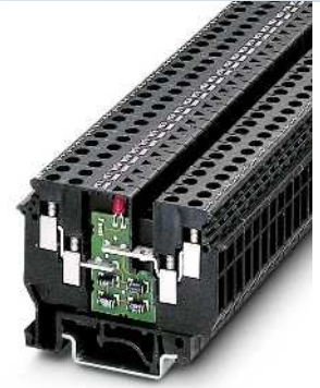
4 (6) mm 2 , 0.5 A, feed-through terminal block, 4 connections, with current indicator up to 1000 mA
