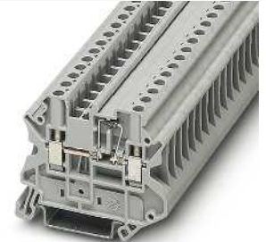
0.5 A, diode terminal block, 1N 4007 (1300 V/0.5 A)
