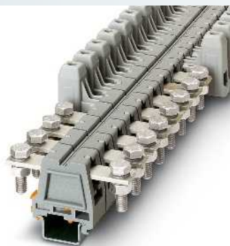
25 (25) mm 2 , 101 A, feed-through terminal block
