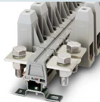
240 (240) mm 2 , 415 A, feed-through terminal block
