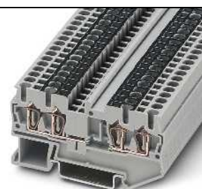
28 A, feed-through terminal block, 4 connections, with interrupted current bar
