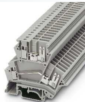
4 (4) mm 2 , 20 A, double-level terminal block with screw and slip-on connection
